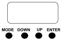
Use MODE to scroll through the available choices. Push ENTER when you reach the option you want to check or set. The current setting for the option will be shown. Use UP and DOWN until you reach the desired setting or menu then push ENTER to invoke the new setting. Use ENTER to exit from the sub menus.
